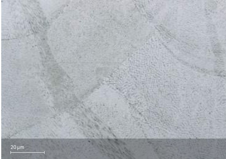
Micrograph etched as manufactured Etchant: ASTM E407-07, etchant 12
