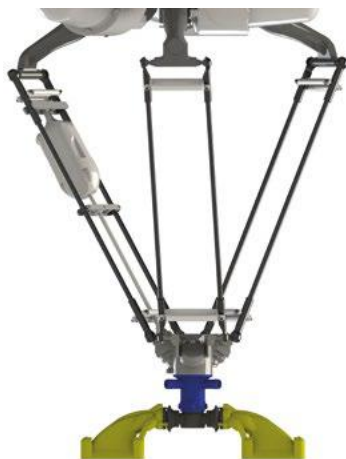
A dual-box version of the completed vacuum assembly, shown attached to a robot. (source: Anubis 3D)
